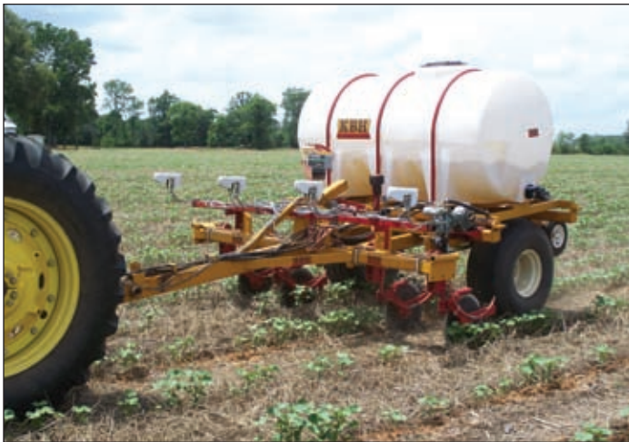
Precision agriculture technologies such as variable-rate fertilizer applicators can increase cotton profitability by improving nutrient use efficiency.
