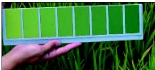
Figure 2. The leaf color chart developed by University of California Cooperative Extension (UCCE) for rice in California.
