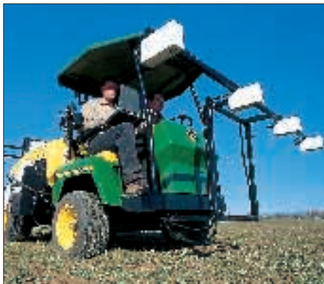
Photodiode based sensors (4 white boxes) collect spectral radiance measurements in the red (660 nm) and NIR(780 nm) regions. Rear nozzles of applicator are capable of applying a prescribed N rate (0 to 100 lb N/A) to each 10 sq. ft., travelling at 10 miles per hour.
