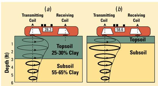
**Figure 1.** EM-38 principle of operation in soils.
