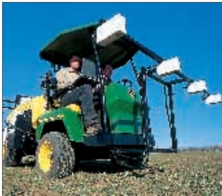
**Photodiode based sensors** (4 white boxes) collect spectral radiance measurements in the red (660 nm) and NIR(780 nm) regions. Rear nozzles of applicator are capable of applying a prescribed N rate (0 to 100 lb N/A) to each 10 sq. ft., travelling at 10 miles per hour.
