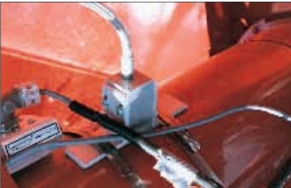
**The sensor** is shown here mounted on a combine during protein and moisture testing.
