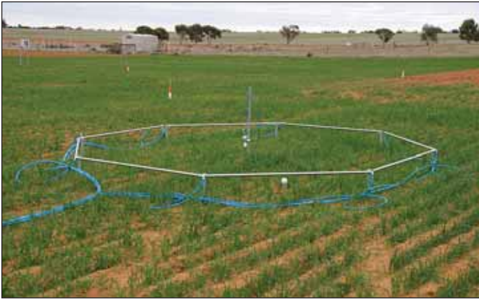
Figure 2. One of the eight free-air CO 2 enrichment rings in the field at Walpeup, Victoria. Eight normal plot areas well spaced from these rings were used as comparisons.
