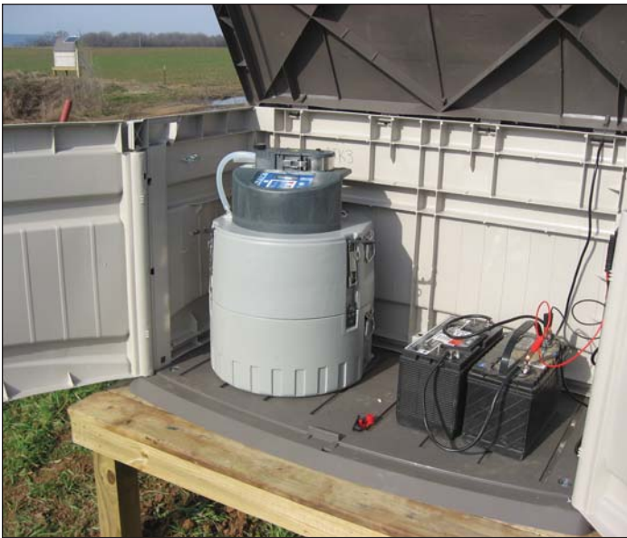
Automated sampler collects water during runoff at Atkins, Arkansas (left) and in-line water flow meter for irrigation water input (right), at Dumas, Arkansas.
