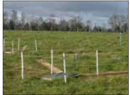
Three surface lysimeters were established at each treatment.
