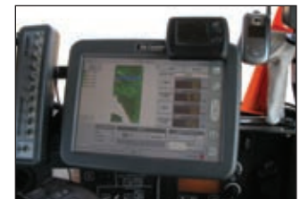
Two-product variable rate application and section control is handled by AgLeader Insight in the tractor cab.
