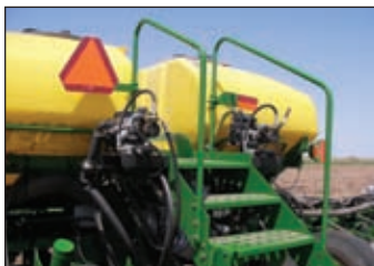
On the Kastens Farms’ planter , two diaphragm pumps (one for 10-34-0 and one for 32-0-0) are hydraulically controlled.
