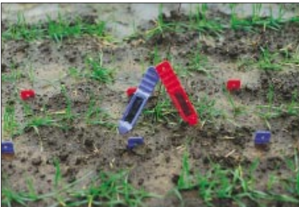
Resin probes used to measure availability of cations and anions in soil solution.
