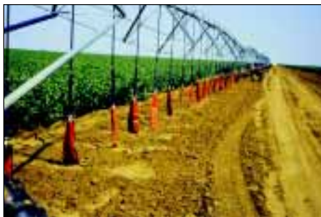
LEPA (low energy precision application) greatly reduces evaporation losses when irrigating cotton.
