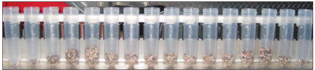
Visual illustration of the resulting distribution from an individual pan test using Blend 1 (17-17-17). Note that the DAP particles (larger in diameter) were applied further out than the KCl (pink particles) and ammonium nitrate (white particles). While not clearly visible, the center three tubes contain the highest percentage of dust particles, which were mainly ammonium nitrate.
