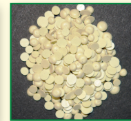
Sulfur pastilles, containing small amounts of clay to enhance dispersion and oxidation
