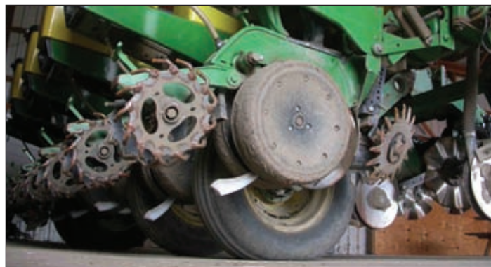
Corn planters for conservation tillage provide the choice of placing fertilizer with or beside the seed, supporting soil-test-based decisions.
