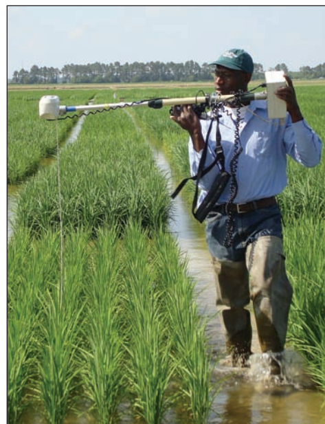
Collecting NDVI readings using a GreenSeeker handheld sensor at panicle differentiation stage at LSU AgCenter Rice Research Station in Crowley, Louisiana.
