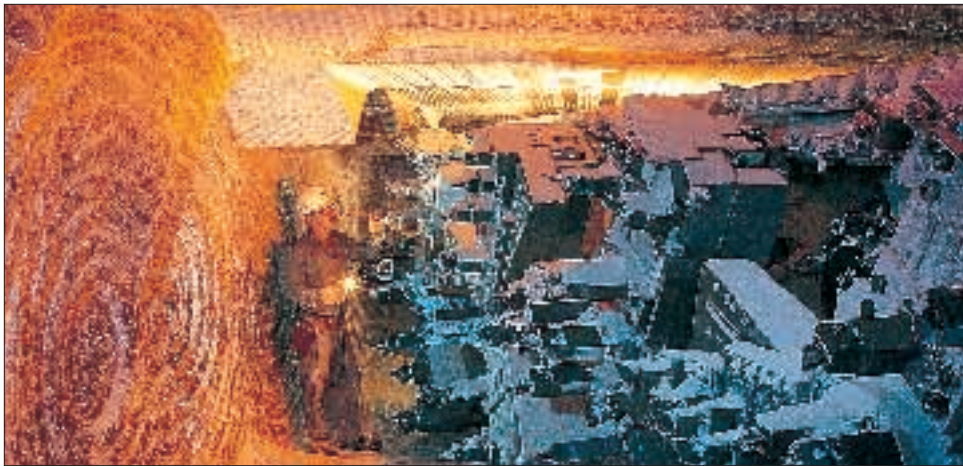
Giant mining machines cut into the potash ore in underground bedded deposits.
