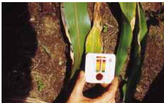
A low cost Pehameter (Hellige) provides a quick pH test in the field.
