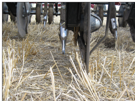
Nitrogen is precision-banded to the side of the seed-row using a coulter-opener.
