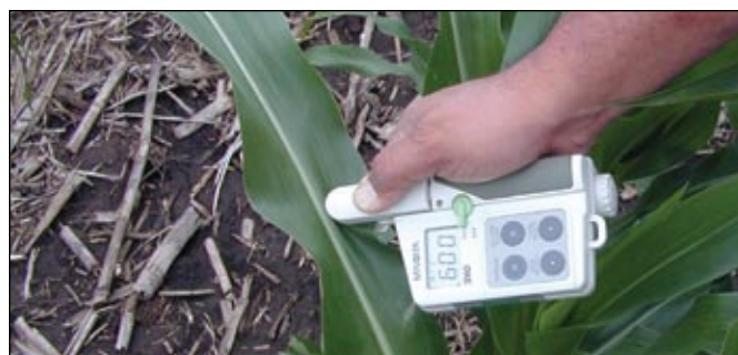
A hand-held chlorophyll meter can be effectively used to guide in-season N application. Photo courtesy of John Sawyer, Iowa State University.
