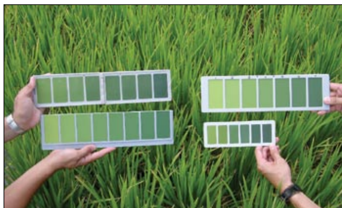
Examples of leaf color charts tested in some regions of the world, such as Southeast Asia for evaluating N needs in rice. Photo courtesy of International Rice Research Institute (IRRI).
